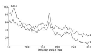
FIGURE 2. X-ray diffraction pattern of pea starch: (a) native, (b) modified.
