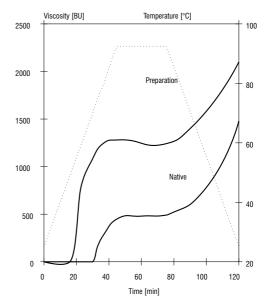
FIGURE 4. Brabender viscosity curves of native and modified pea starch.
