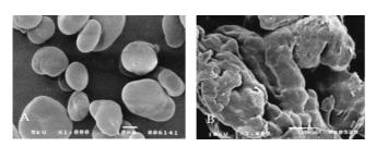
FIGURE1. Microstructure of native pea starch (A) and its preparation (B).
